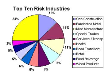
General Construction is associated with the highest number of injury at all levels of severity as well as the highest number of fatalities. Most cases occurred during demolition work.
