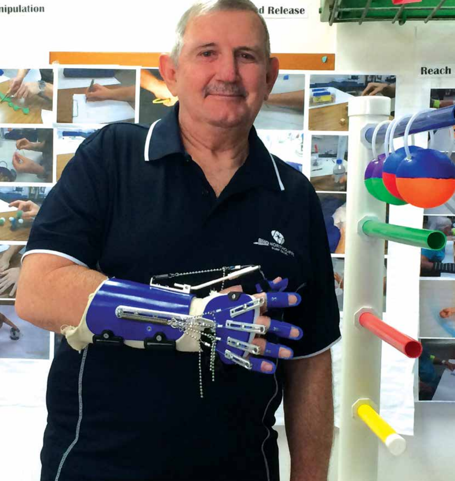
Above: Recovering stroke patients like Russ Noyes have a new device to help them work on regaining control of their hands. A mechanical arm allows him to incorporate hand functionality in therapy and at home by supporting the weakened wrist, hand, and fingers.
